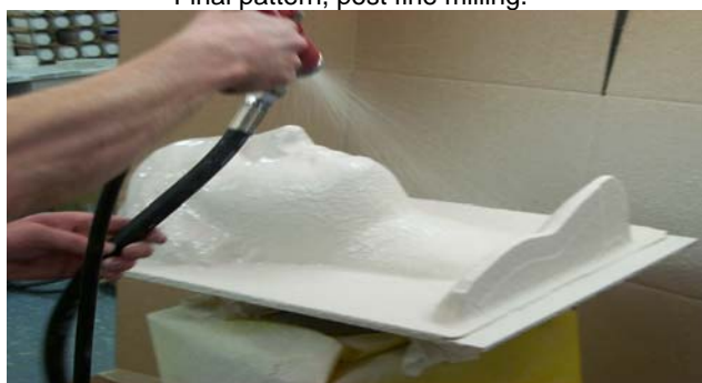
Hand finishing, M2 coating over EPS.
