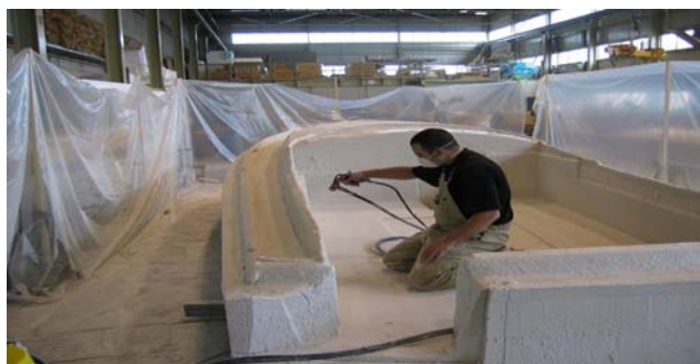
Spraying 20mm over rough milled EPS boat deck.
