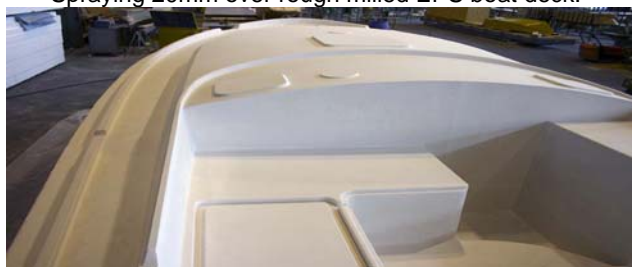
Final pattern, post fine milling.
