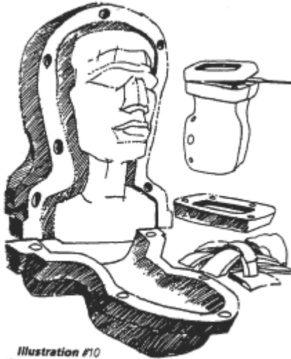
Illustration #10 (Steps 21 through 24) Disassembling the mother mold
